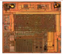
Same idea than with software RE (from binary, to assembly and to code), chips RE go from silicon, to images, to transistors, to gates, to netlist and to algorithm.
