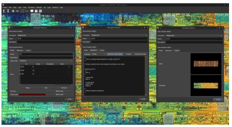
Each identified gate (from the gate library) can be matched manually or using template matching algorithms.
