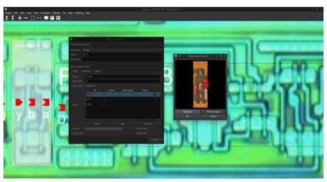
Each gate can be described with VHDL/Verilog, have a list of port (placed on image), a type associated etc.
